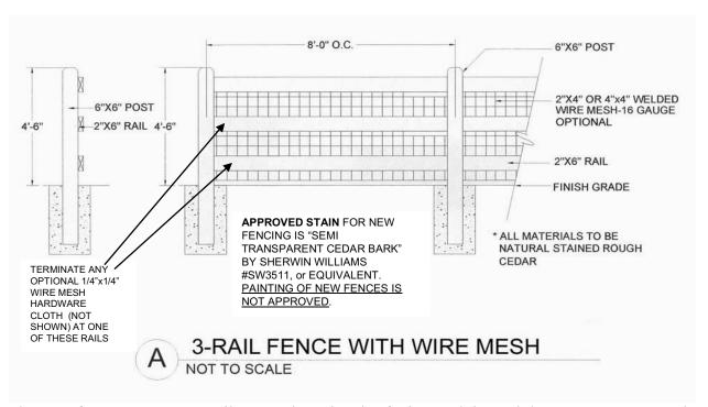
The use of wire mesh on 3-Rail Fences is optional. If wire mesh is used there are two approved types and configurations. Either of the wire mesh configurations described below may be used either by themselves or in combination. Uncoated non-colored standard wire mesh is the only approved color for the wire mesh.
